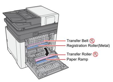
Wipe away the paper dust on the registration roller and the paper ramp using the cloth.
